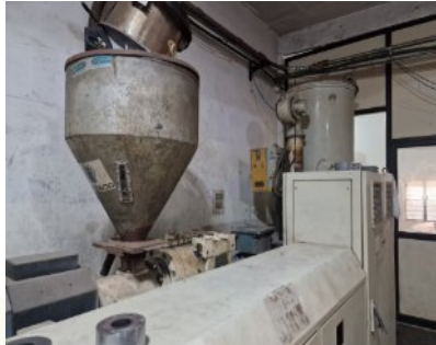
A decommissioned production plant of the Israeli company NetaFim. Granules are filled in.
