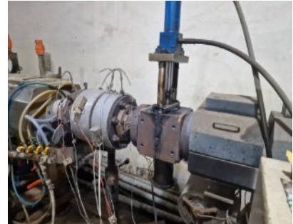
The molten granulate is pressed into a tube shape using high pressure.
